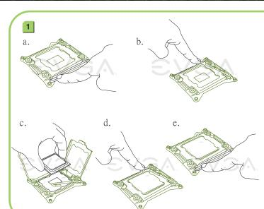
Unhook the left socket lever by pushing down and away from the socket.
