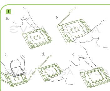
Unhook the left socket lever by pushing down and away from the socket.
