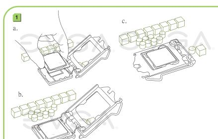
Pull the socket lever back and the load plate will automatically lift.
