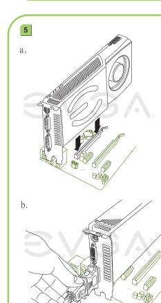
Insert your graphics card into the PCI-E 2.0 slot . The type of slot depends on the graphic card bus type. Connect a monitor to the output connector of the graphics card.
