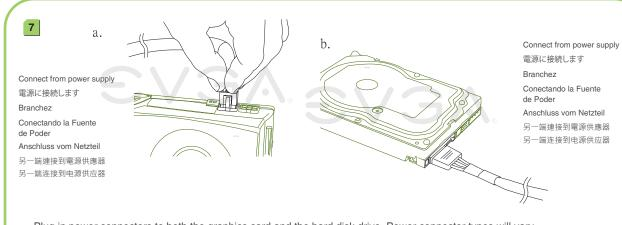
Plug in power connectors to both the graphics card and the hard disk drive. Power connector types will vary depending on the hard disk drive and graphic card's power requirements.
