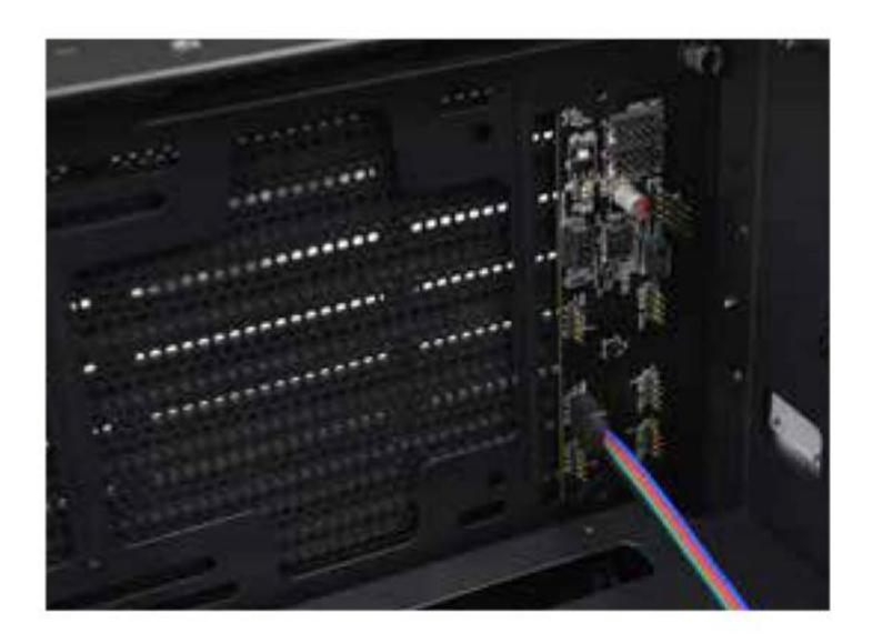
This control board features headers for up to six (6) RGB fans. Please make sure to provide power to the control board by connecting a SATA power cable from your power supply to the control board. You will not be able to control the lighting through the DG-7 if power is not connected. Connected fans can be controlled through the DG-Tuner software, shown below on Page 10.
