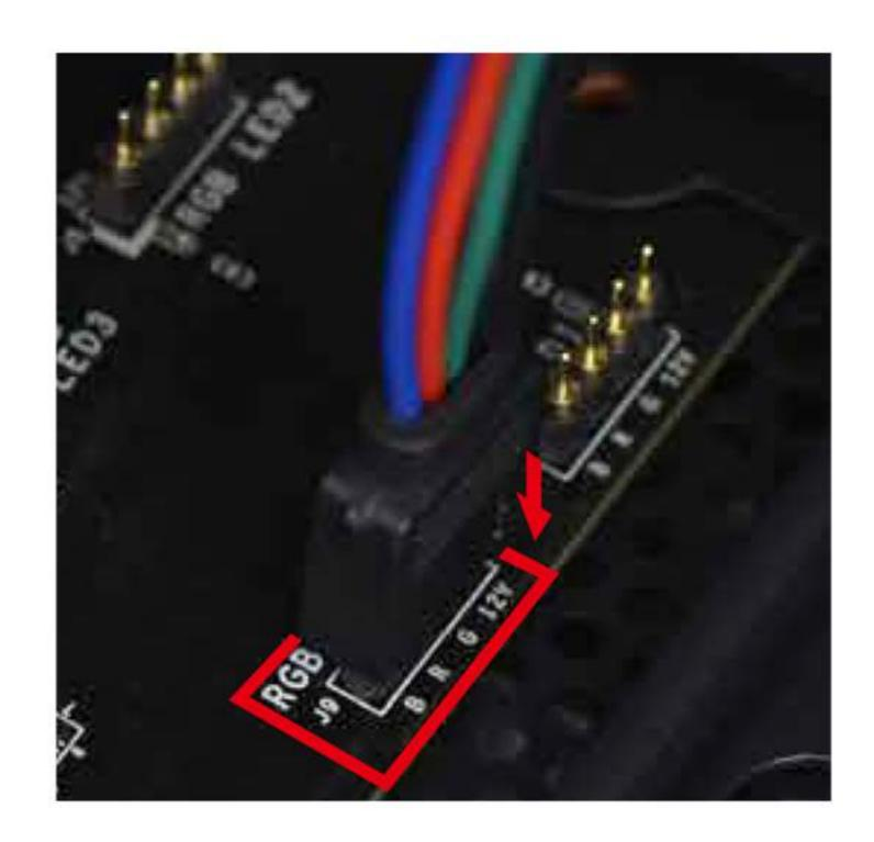
Please note that RGB LED fans use a type of connector that must be correctly installed for the lighting to be properly controlled. Failure to install your cable properly will prevent the fan lighting from working or being controlled.
