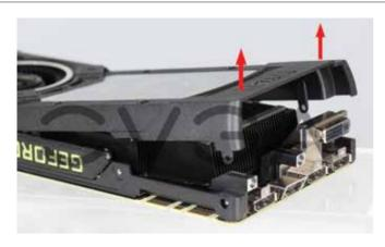
5) Now remove the heatsink and set it aside. We suggest cleaning the bottom of the heatsink, as the thermal compound left there can smear and spread.
