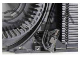
13) The secondary 3 pin cable from the waterblock powers the fan for the radiator. Attach it, and for ease of cable routing, you can use the included ties to attach the cable to the hose.
