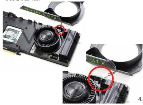
12) Unplug the power for the existing fan plug in the waterblocks pass through power cable into the cards power header, then reattach the fan to the card via the pass through. Make sure the wires do not touch the fan; please use included strips of tape to attach the wires to the plastic around the perimeter of the fan.
