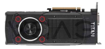
4) Remove the 4 screws on cover, then remove the left cover (1.5mm hex bit).
