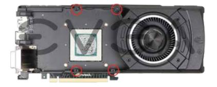
9) Be sure to clean the GPU (see pic) with alcohol (preferably 90%) removing all thermal compound.
