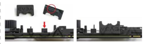
11) Remove the plastic cap on water block, use the 4 Spring Screws previously removed to mount the block on the GPU (Thermal compound is pre-applied to the block).
