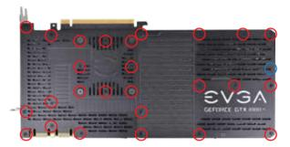
2. Remove heatsink and fan, while carefully disconnecting fan and LED connectors.
