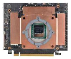
(b) Please check to make sure that your thermal pads are in the same location as photo below. If not, please check the back of the card in case the matching thermal pad remains on the card. Install the memory baseplate, as shown in Step 4(a). Hold the copper plate in place and turn the card over. Place the right backplate over the card and tighten the backplate with 4 #8 screws, as shown in the left photo below.
