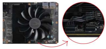
(a) Prepare #1 Shroud by removing any adhesive film, and locate the two LED connectors.
