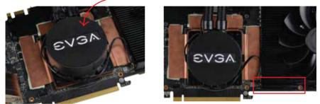
(c) Plug the pump's power connector into the left fan header, as shown in the photo below. The Y-cable will remain unused. Make sure to flatten the cable to be level with the heatsink, to avoid contact with the fan.
