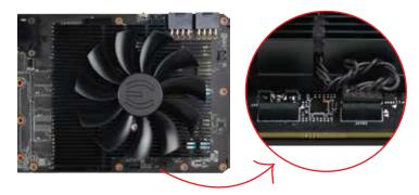
(b) Please check to make sure that your thermal pads are in the same location as the photo below. If not, please check the back of the card in case the matching thermal pads remain on the card. Carefully turn the graphics card over while holding the heatsink in place. Avoid tilting or putting direct pressure on the fan. Plug in the backplate's LED connector to the matching connector on the graphics card, as shown in the left photo below.
