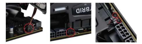
(c) Install the shroud over the PCB. Make sure to slide the shroud under the edge of the PCI bracket, as shown in the left photo below. Once the shroud is in place, tighten 2 #7 screws in the area circled in red, as shown in the right image below.
