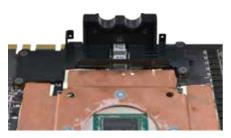
(b) Tighten 3 #08 screws in the circled areas, as shown in the photo below.
