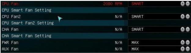
ALL FAN HEADERS ON THIS MOTHERBOARD HAVE A MAXIMUM POWER LIMIT OF 1 AMP @ 12 VOLTS, OR 12 WATTS, ANY MORE THAN THIS WILL LIKELY DAMAGE THE BOARD AND CAUSE PERMANENT FAILURE OF THE FAN HEADER. IF YOU NEED TO RUN A HIGH CAPACITY FAN, OR A PUMP THAT PULLS MORE THAN 1 AMP/12 WATTS, PLEASE USE A MOLEX CONNECTER FROM YOUR POWER SUPPLY, OR IF CONTROLLING THIS DEVICE IS NECESSARY, PLEASE LOOK TO A FAN CONTROLLER.
