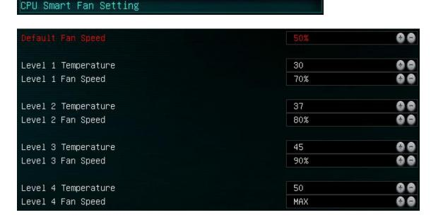
This is an example of a fairly aggressive fan curve, but not uncommon for overclocking or running in a warmer environment. At each Temperature Level you can manually enter any value in Celsius you want then below set what speed you want the fan to run at.
