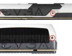
3) Remove the 4 spring screws on the back side of the card (#1 Philips Bit) this will allow the heatsink
