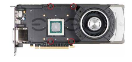
14) Attach the shroud to the card, you can use the hoses and the fan as alignment marks. It will use the 8 bolt holes the original shroud used. Please use the included screws for the new shroud. (#1 Philips bit)
