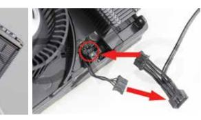
13) The secondary 3 pin cable from the waterblock powers the fan for the radiator. Attach it, and for ease of cable routing, you can use the included ties to attach the cable to the hose.
