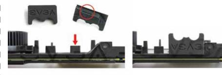
11) Remove the plastic cap on water block, use the 4 Spring Screws previously removed to mount the block on the GPU (Thermal compound is pre-applied to the block).
