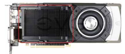
6) Remove the 4 screws holding the center portion of the shroud, and remove it. (#000 Philips bit)
