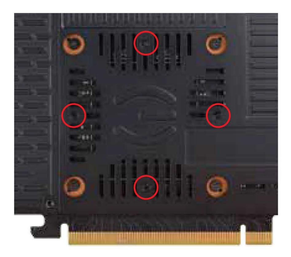
(b) Apply thermal grease to the GPU when you are ready to install the waterblock. There are many different ways to correctly apply thermal grease, so please use the photo below as a reference for how much to apply. Take care to avoid putting thermal grease on any other components. If you do get thermal grease on other components, clean any affected areas with high percentage isopropyl alcohol and a lint-free cloth or cotton swabs prior to installation of the waterblock.
