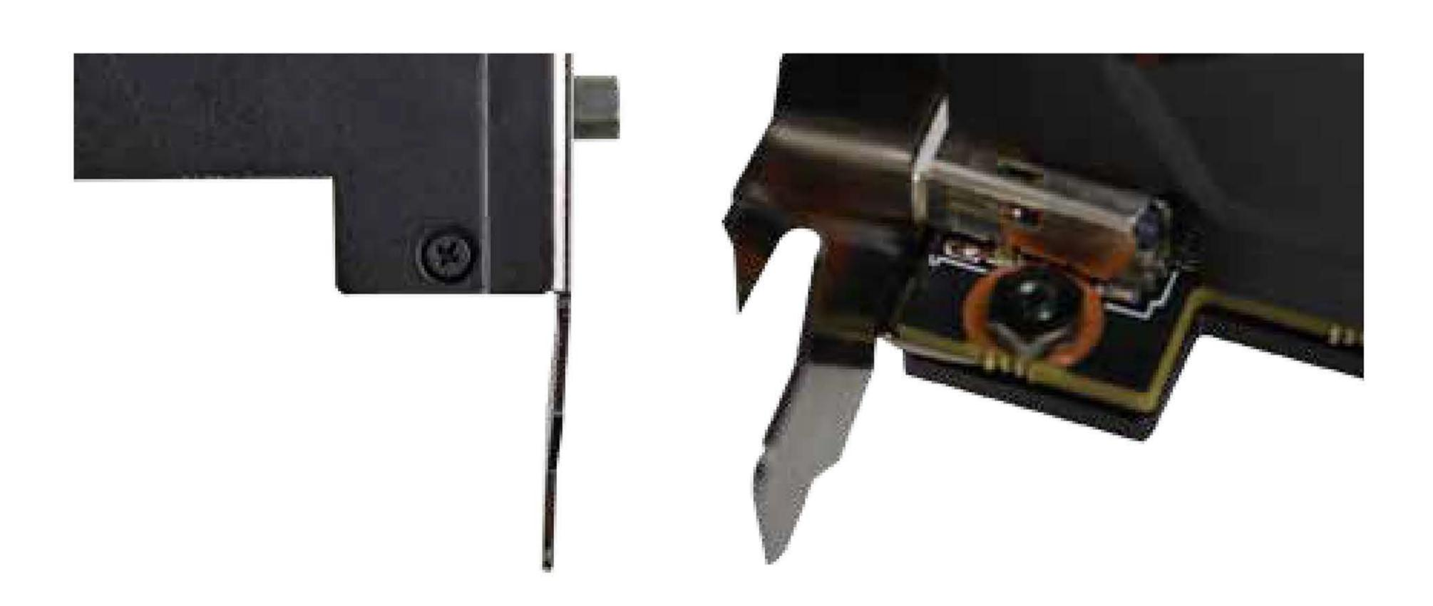
At this point, your waterblock should be fully tightened and ready to test. As noted before, please use care to avoid overtightening, as this may strip the screws and/or damage the graphics card. Lastly, do not use power tools to install the waterblock or backplate.
