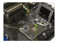
Align notches with notches on the CPU
