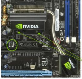
The nForce SPP and MCP have a passive heat sink that draws heat from the chips. You can install a fan onto the SPP heat sink that helps to cool the chips. Hook the fan over the SPP heat sink. Use the two screws to secure the fan to the SPP. Plug the cable into the fan connector.
