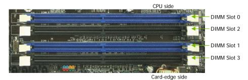
Use the following procedure to install memory DIMMs into the slots on the motherboard. Note that there is only one gap near the center of the DIMM slot. This slot matches the slot on the memory DIMM to ensure the component is installed properly.
