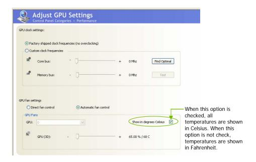
Figure 20. Adjust GPU Settings (nTune)
