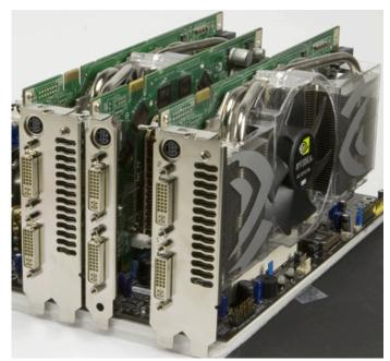
Three PCI Express graphics cards installed. Only the two outer cards will be SLI'ed using the SLI Connector shipped in your motherboard kit.
